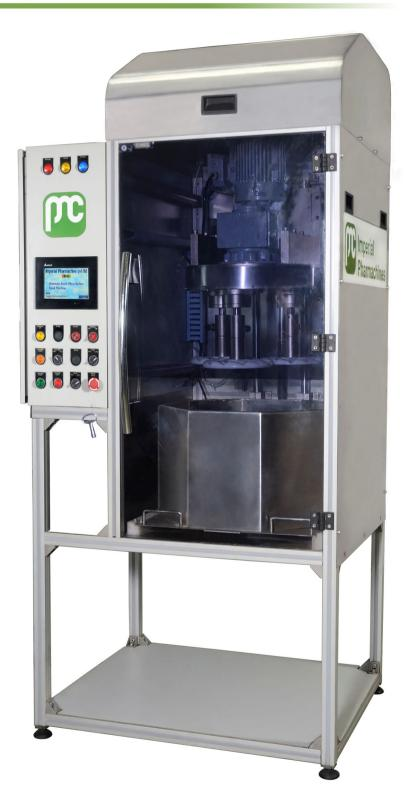
Auto Punch Polisher helps improve the surface finish of punches, which leads to improved tablet finish, minimises sticking and prevents corrosion.
